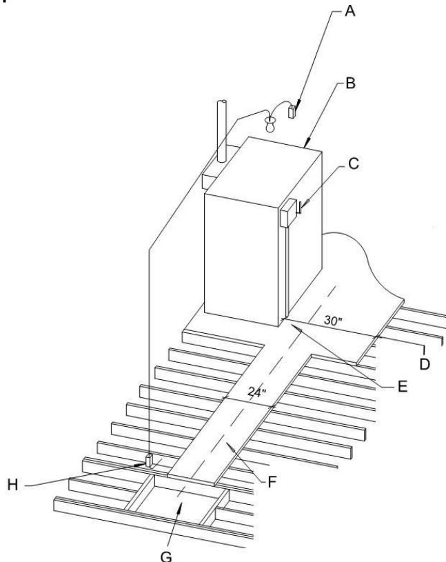
**Trusses:** Where trusses are used as attic floor framing, they shall be designed for load bearing.
