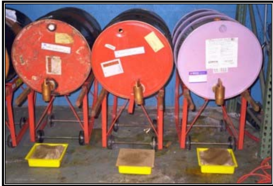
Figure 4.18. Mounted Containers with Drip Pans.
