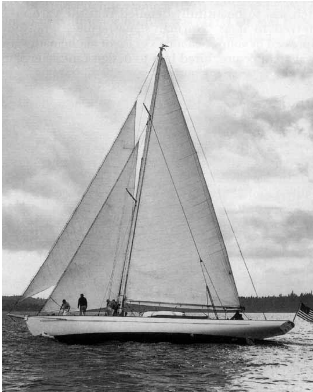
The CIRCE, launched by Ben Seaborn at age 17. The boat originally measured 54' and was later lengthened to 63'. Photographer: Ray Krantz. Source: Bunnell, Steve. (May/June 1999). Wooden Boat , No. 148. "Shooting Star: The Tragically Short Career of Ben Seaborn," p. 77.
