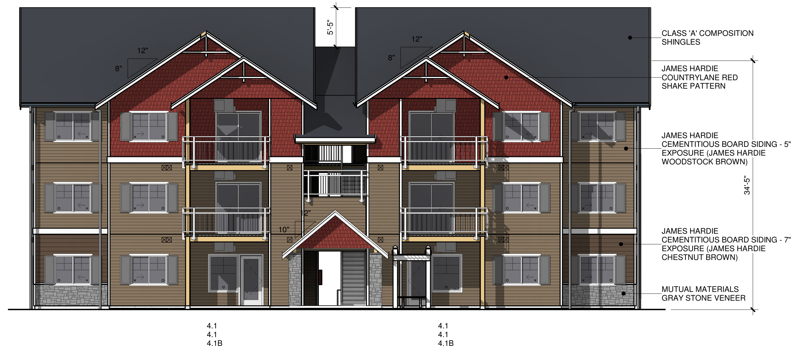
BUILDING 'D' - FRONT ELEVATION - NORTH
