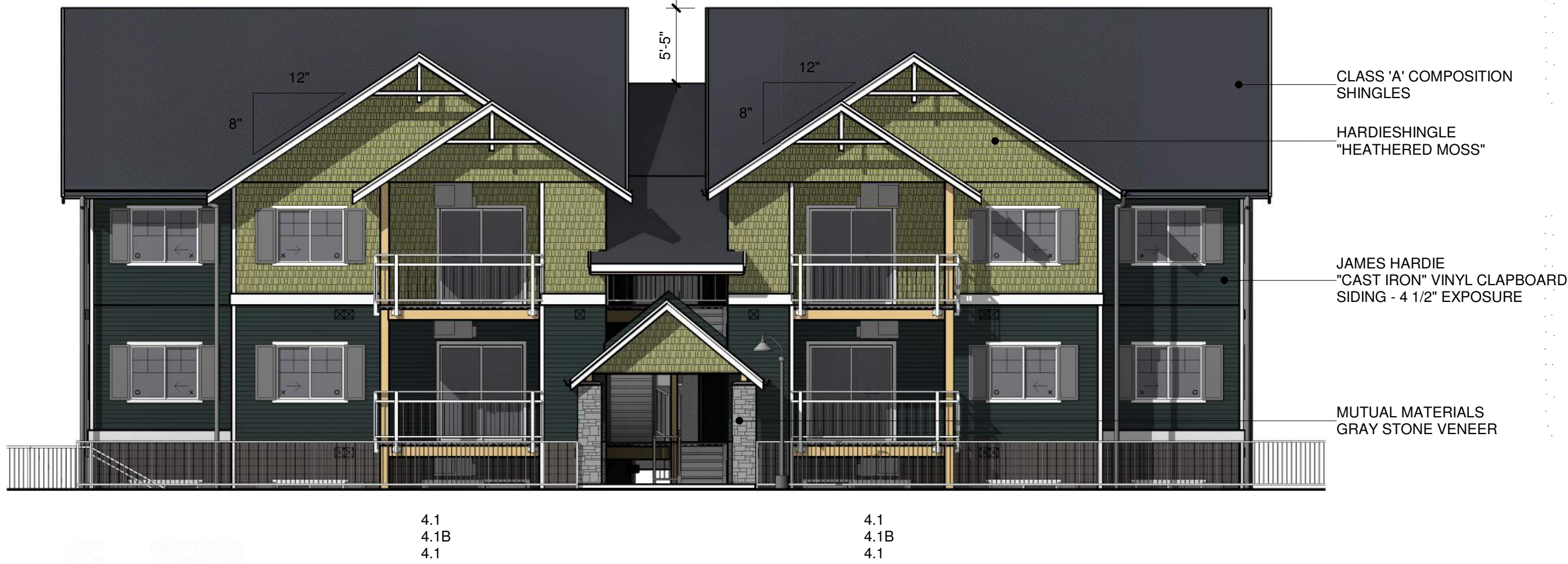
BUILDING 'C' - FRONT ELEVATION - NORTH 1/8" = 1'-0"
